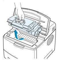
With a dry and lint-free cloth, wipe away any dust and spilled toner from the toner cartridge area and the toner cartridge cavity.
